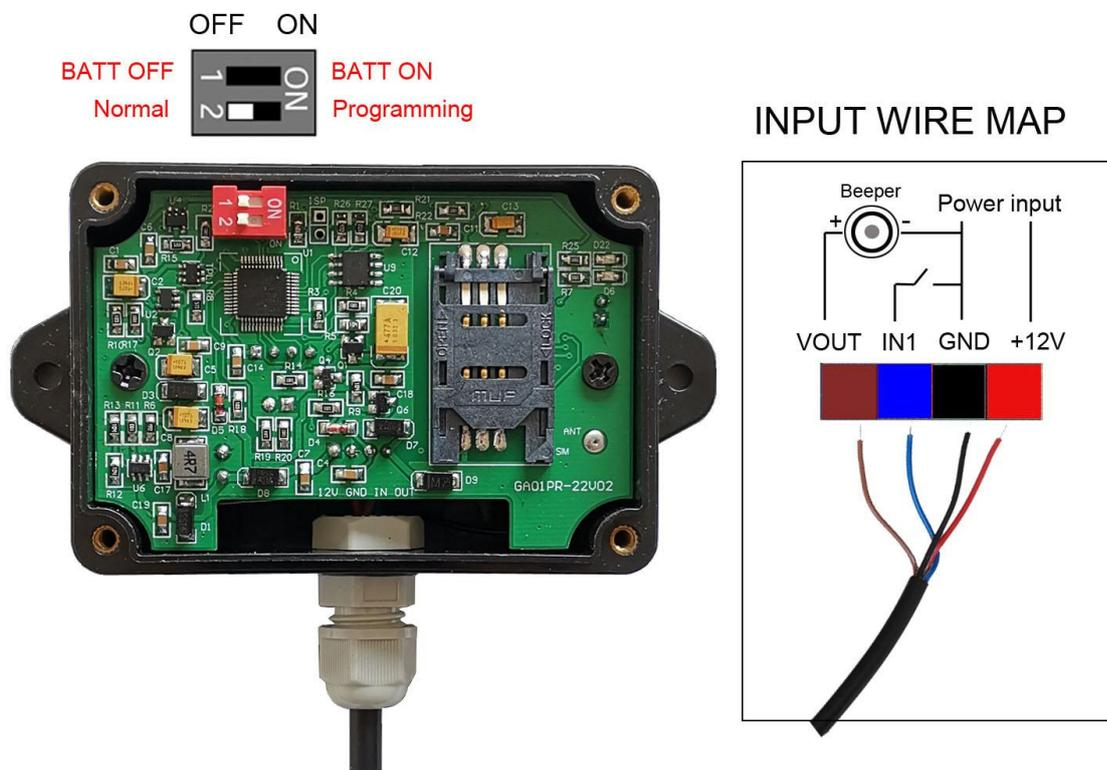
When IN1 input is shorted to GND, then will trigger the alarm
