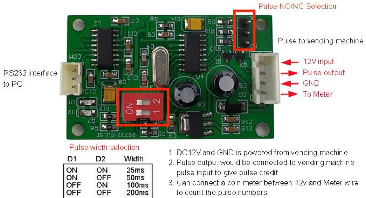
**It must be noted that the “Pulse” and “Meter” outputs must not be short-circuited with “12V input”, as this will cause permanent damage to the output components. Therefore, before testing, be sure to wire carefully and bandage separately.**
